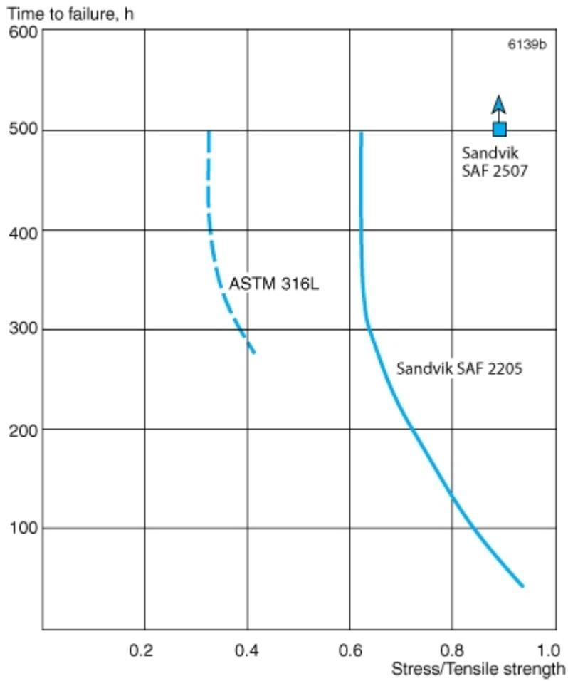
Figure 14. Results of SCC tests with constant load in 40% CaCl<sub>2</sub>, pH=1.5, at 100 °C (210°F) with aerated test solution.
