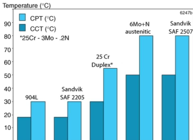
Figure 10. Critical pitting and crevice temperatures in 6% FeCl<sub>3</sub>, 24h (similar to ASTM G48).
