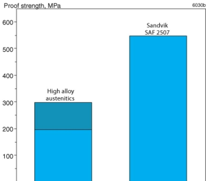
Figure 1. Comparison of minimum proof strength, 0.2% offset, of SAF 2507® and high alloy austenitic grades, for material in the solution annealed condition.
