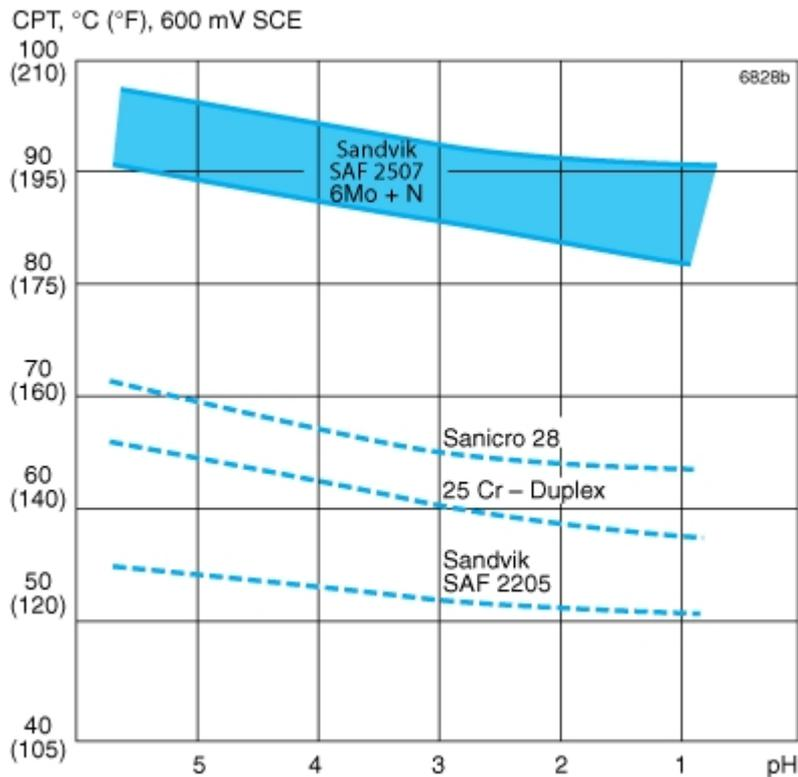
Figure 12. Critical pitting temperatures (CPT) in 3% NaCl with varying pH (potentiostatic determination at +600 mV SCE with surface ground with 600 grit paper).
