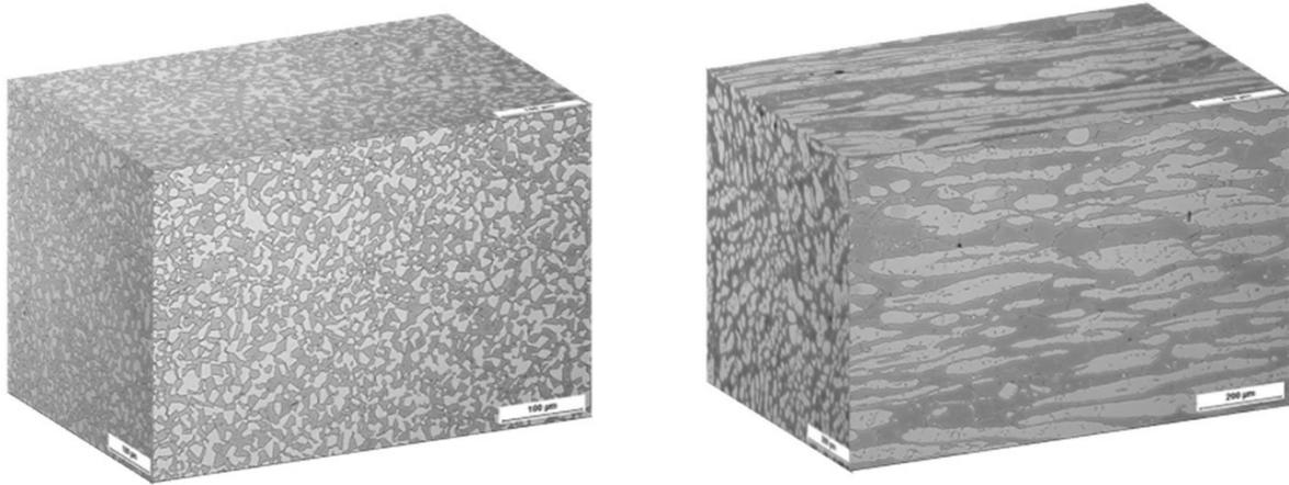
Fine isotropic microstructure of HIPed material vs. forged bar. Note micrographs show duplex material for illustration.
