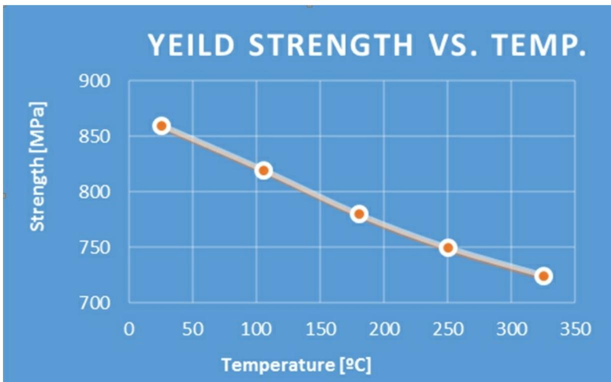
The mechanical properties of APM 9980 can be customized in a wide range by varying heat treatment. If properties listed here does not meet your requirements, please contact Sandvik Powder Solutions for more information.
