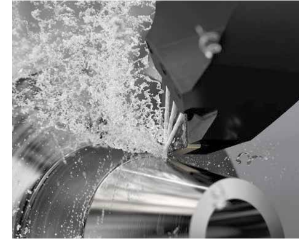
Machining of Sanicro® 825 nickel alloy bar using Sandvik Coromant carbide cutting tool.
