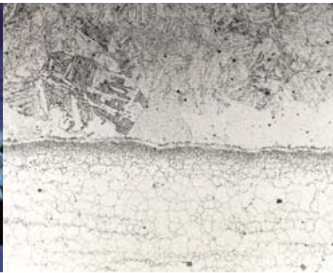
Figure 6, left. Bonding zone in a composite tube Sandvik Sanicro 28/HT7 (Sandvik Sanicro 28 on ASTM A213/T91). The Sanicro 28 component is shown at the top of the figure.
