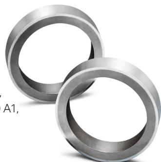
Figure 2. Sandvik composite tubes consist of two different materials metallurgically bonded together through hot extrusion. By selecting the correct alloy for the outside and inside component, the corrosion resistance and the mechanical properties are optimised and a tube that meets conflicting material requirements inside and outside is obtained.
